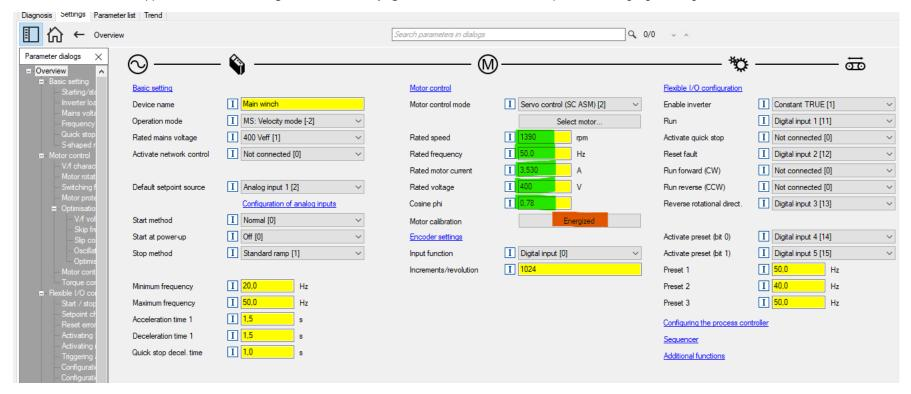
Then perform the motor self-calibration by clicking "Energized" (highlighted in red))
