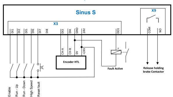
Reference wiring diagram control section
