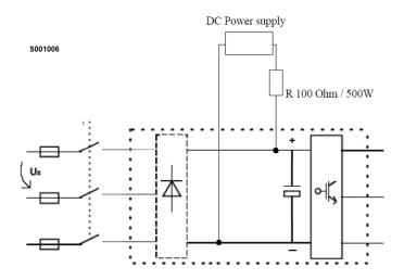
Figure 3. The reforming circuit for method 2B.
