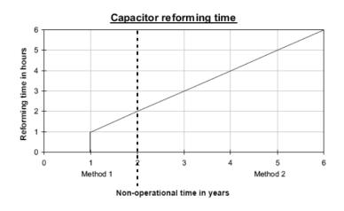
Figure 1. Capacitor reforming time.
