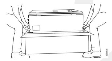
All the parallel string boxes must be installed in upright position. To facilitate installation, the parallel string boxes come supplied with special brackets.
