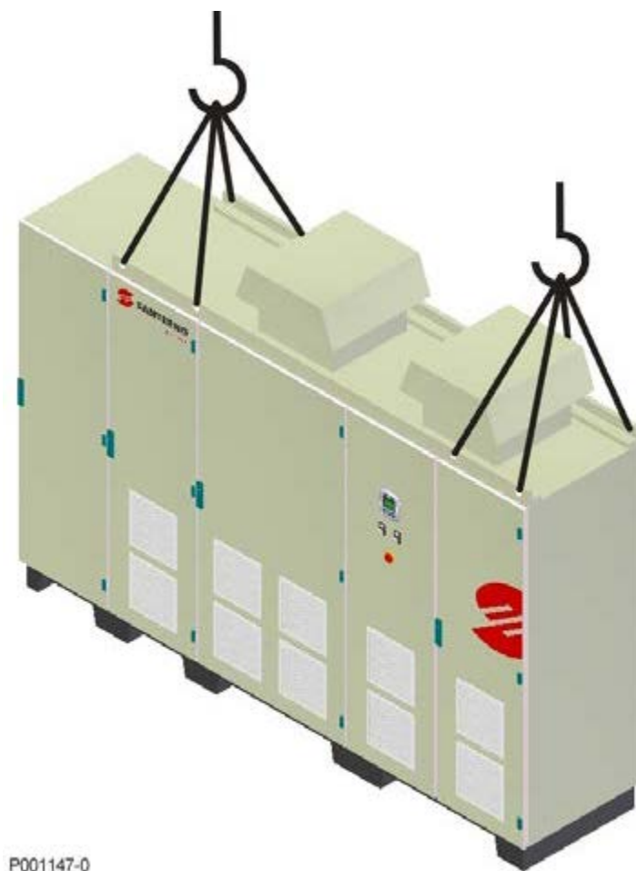
Figure 5: Correct hoisting of inverters
