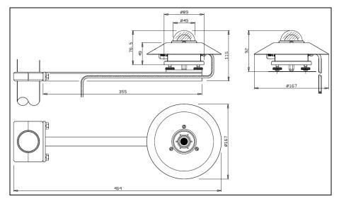
Figure 19: First class pyranometer
