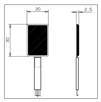
Figure 20: Contact temperature sensor
