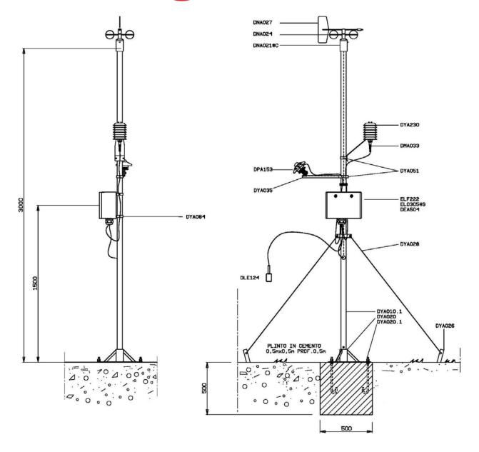
Figure 2: Components of the Meteo Center weather station
