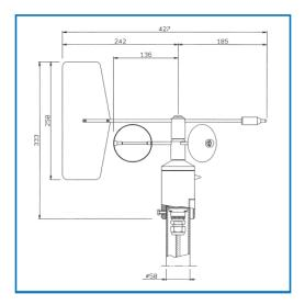
Figure 18: Wind direction and wind speed combined sensor
