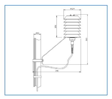
Figure 17: Air temperature sensor
