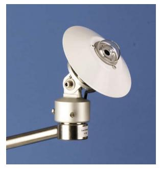
Figure 6: First class pyranometer
