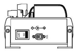
Figure 9: Power supply connector
