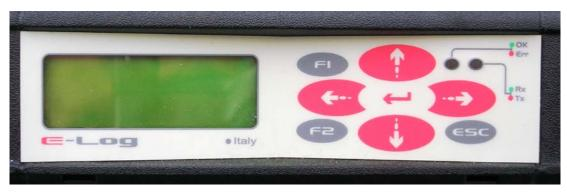
Figure 14: Front part of the datalogger
