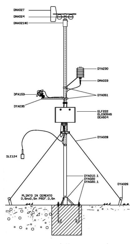
Figure 8: Positioning the Meteo Center on a pole
