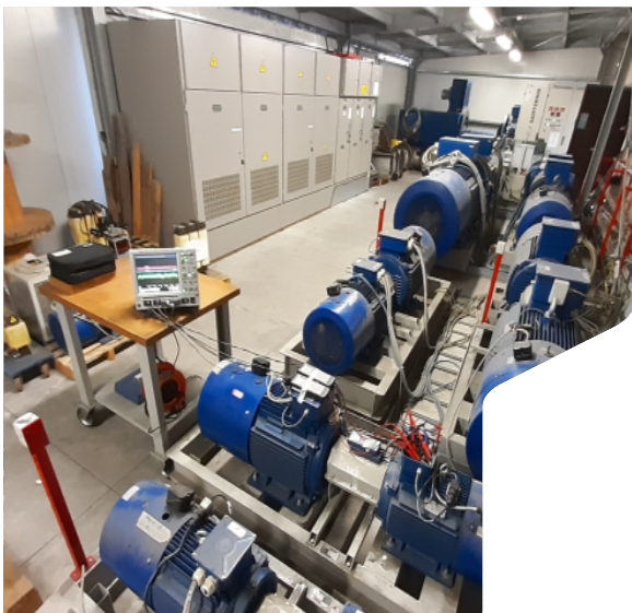
Figure 3 – electrical motors room with motor-brake pairs, powers ranging from 10 to 800 kW
