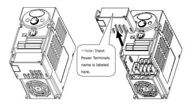
To access control terminals: after finishing power terminal wiring, reinstall the bottom cover and then start wiring control terminals.
