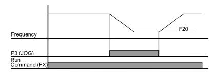
Jog operation overrides all other operations except Dwell operation. Therefore, if Jog frequency command is entered in the middle of Multi-Step, Up-Down or 3-wire operation, operation is executed at Jog frequency.
