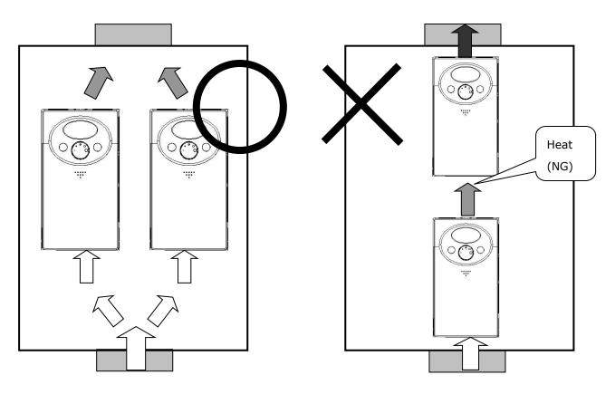
Note: Take caution on proper heat ventillation when installing inverters and fan in a panel.
