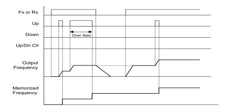
▶ When F65 is 2: It is increased as much as step frequency set as F66 at the rising edge of multi-function input set as UP and if it is activated for 3 seconds, it operates as it was set as "0". It is decreased as much as the step frequency set as F66 at the rising edge of multi-function input set as DOWN. If it is activated for 3 seconds, it operates as it was set as "0" and the accel/decel time is the same as when set as "0".
