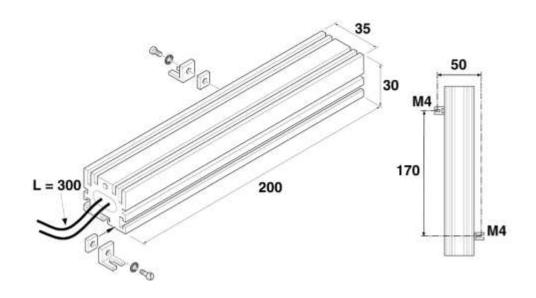
Overall Dimensions, Resistor 350W - IP55
