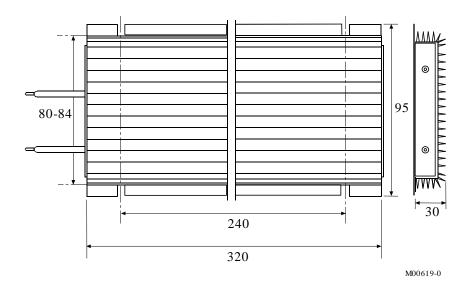
Overall Dimensions, Resistor 1100W - IP55
