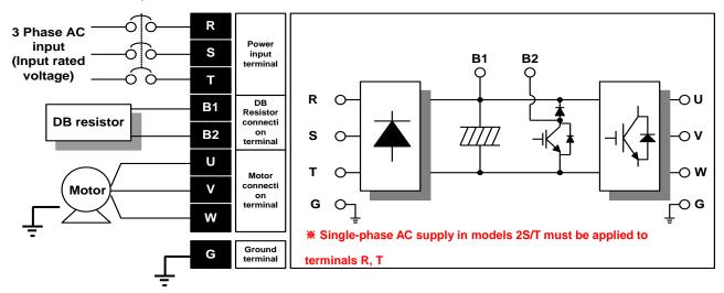
Power terminal wiring (11.0 ~ 22.0kW)
