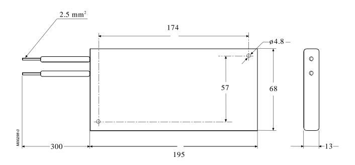
Overall Dimensions, Resistor 550W - IP55
