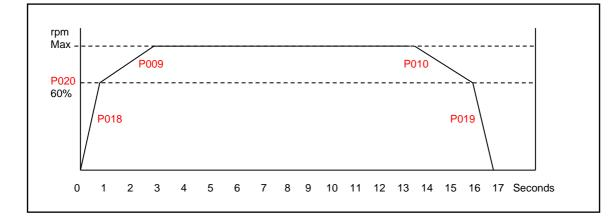
If the plant is at risk of mechanic shock in the pipe lines (water hammer), the ramp time P010 must be extended as much as necessary to reduce or eliminate the shock.
