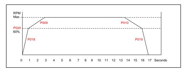
If the system is at risk of mechanic shock in the pipe lines (water hammer), the ramp time P010 must be extended as much as necessary to reduce or eliminate the shock.
