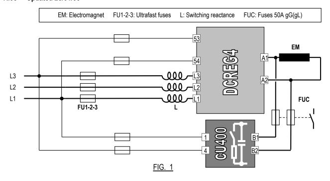
**Otherwise**, if you suppose that over voltage occurs only when the conduction mesh opens on mains side (3-phase supply voltage L1-2-3 derived from sliding brushes), another protective measure exists.
