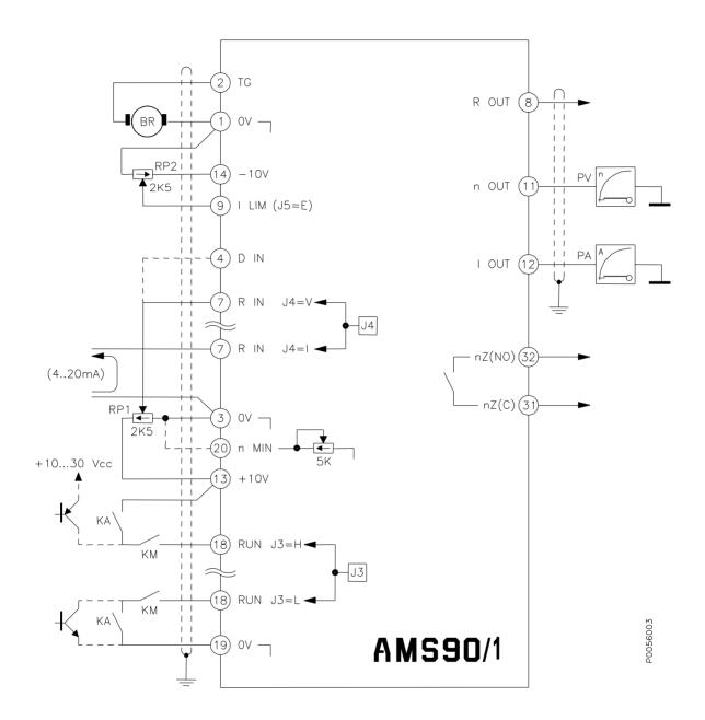
Note: to have the drive match the standards concerning radio-frequency immunity characteristics, keep 0V of the board (term. 1-3-19) insulated from earth. In turn, connect cable shield to the earth, through a connection that should be as short as possible.
