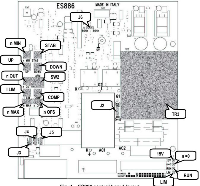
Fig. 4 - ES886 control board layout
