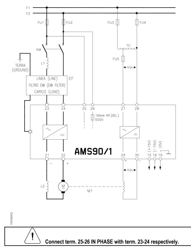
Fig. 2 - Power and supply connections diagram
