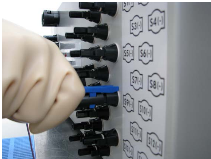
Figure 30: Disconnecting a string connector
