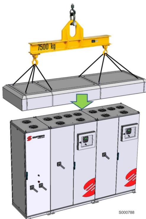
Figure 23: Placing the rooftop on the inverter
