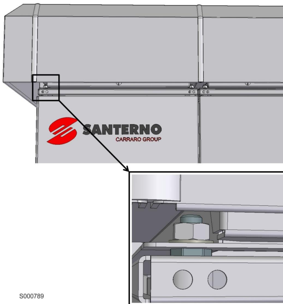
Figure 24: Fastening the rooftop to the inverter
