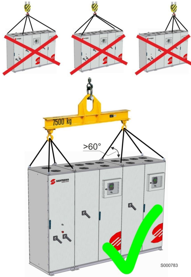
Figure 17: Hoisting the inverter (TG1200 1000V TE, TG1800 1500V TE)
