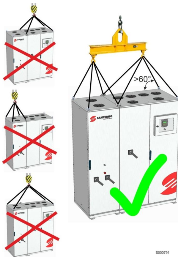
Figure 18: Hoisting a 3-door inverter
