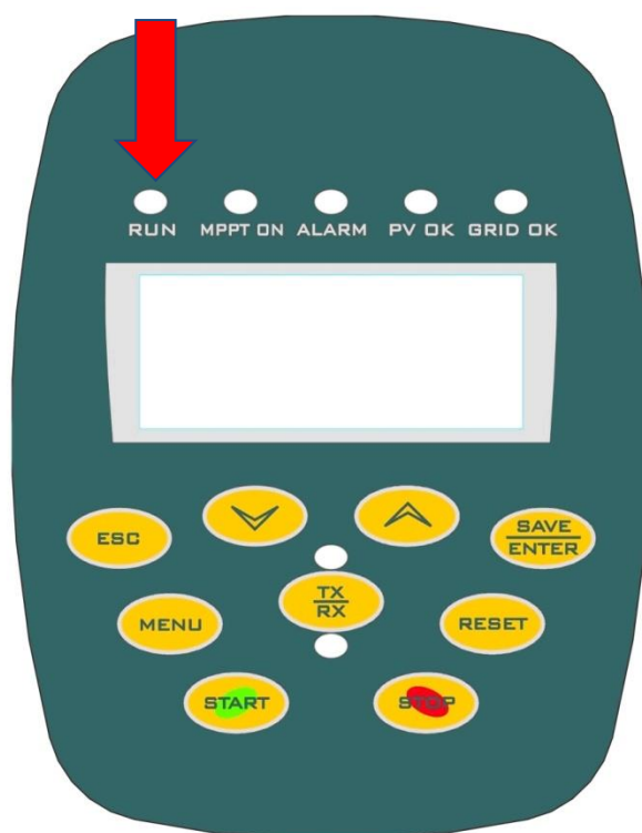
Figure 8: RUN LED on the display/keypad
