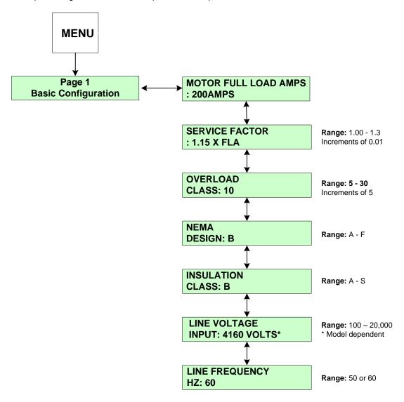
**SP1.1 Motor Full Load Amps (FLA):** Allows the user to enter the motor's FLA rating. Range of adjustment is 50 - 100% (less programmed service factor).
