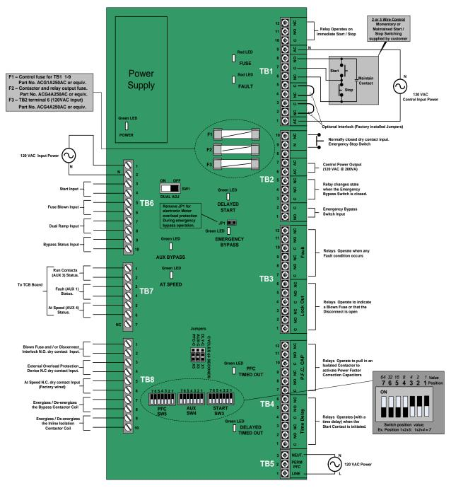
FIG. 2.2.1 TCB Terminal and Control Board
