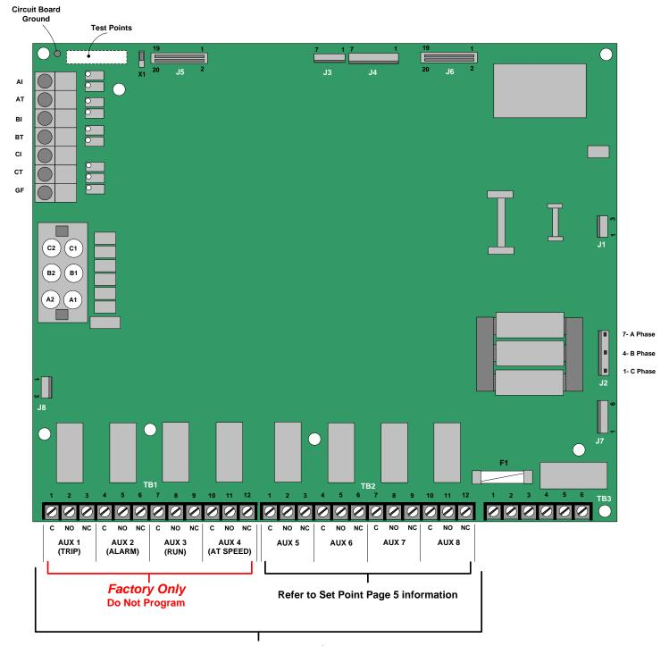
Relay Output Contact Rating: 240VAC @ 5A (1200VA)
