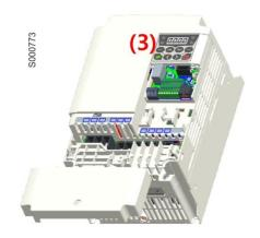
■ Unfasten a screw from I/O board and fasten the prepared brass bar (4) and (5).
