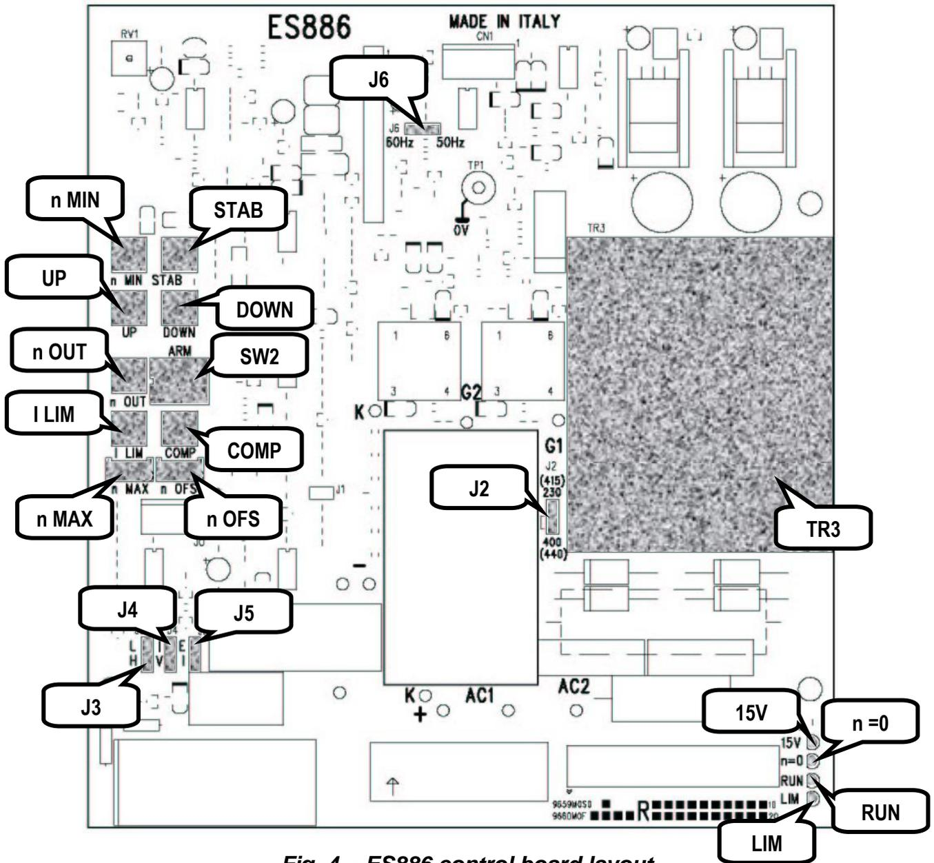
Fig. 4 - ES886 control board layout
